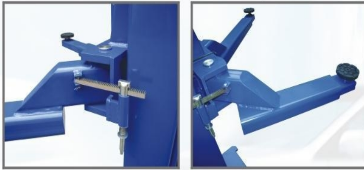
The arm is credible locking structure. Adopt un-symmetry arm.
